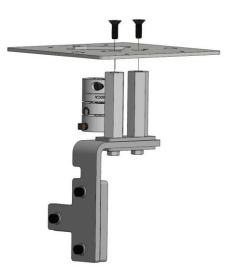
Figure 5: Attach Actuator Bracket
