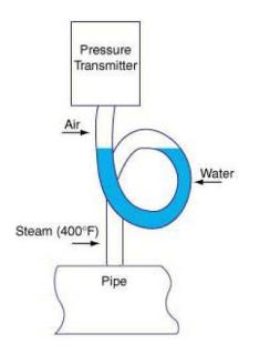
Figure 1: Example of a Syphon Loop
