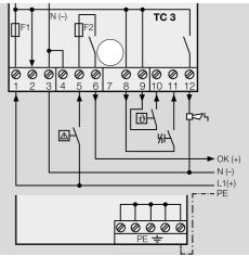
Mains voltage: 120 V AC/230 V AC, control voltage: 24 V DC
