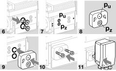
→ Tighten the screws with max. 250 Ncm.
