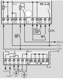
Mains voltage: 120 V AC/230 V AC, control voltage: 24 V DC
