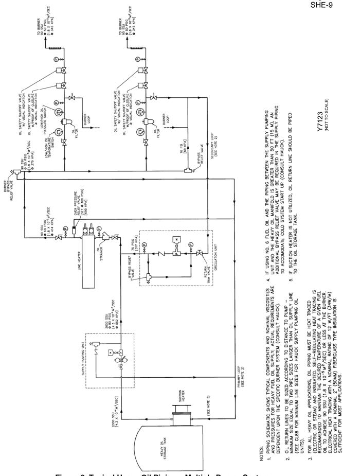
Figure 2. Typical Heavy Oil Piping – Multiple Burner System
