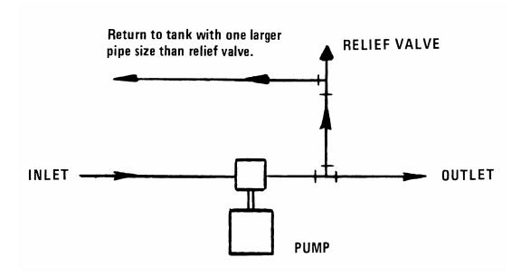
Fig. 2 - Typical piping arrangement showing pressure relief valve placement.
