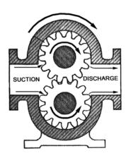
Figure 3. Proper Oil Flow Through Gear-Type Rotary Pump.
