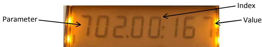
Figure 7-1: LME7 Fault History Example with Indexes
