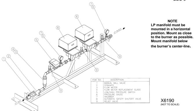
Figure 8. PLPM Prepiped LP Manifold Detail
