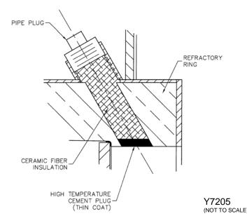
Figure 5. Alternate Port Sealing Instructions
