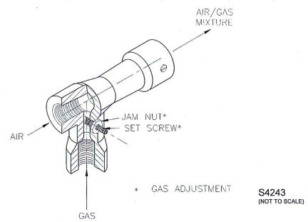
Figure 2. Pilot Mixer Adjustment
