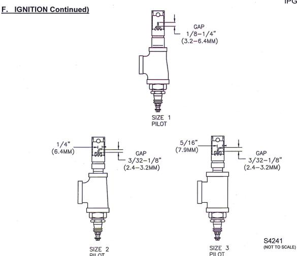
Figure 1. Spark Gap Setting and Electrode Positioning
