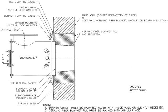
Figure 2. Burner Installation With Alloy Tile
