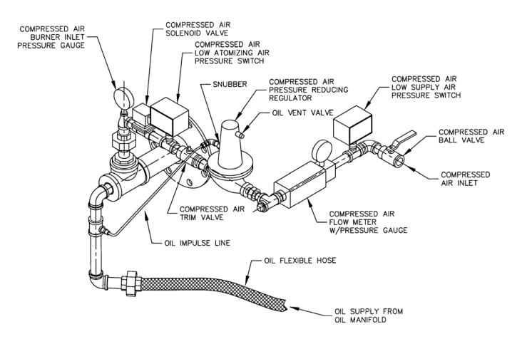
Figure 11. Compressed Air Manifold Detail
