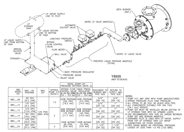
Figure 7. Typical Schematic of LP Supply Piping
