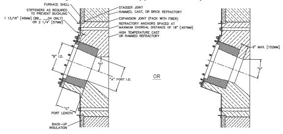
INSTALLATION DETAIL SHOWN TO EMPHASIZE BURNER TILE/PORT GEOMETRY. FURNACE WALL SHOWN AS 'TYPICAL' REFRACTORY CONSTRUCTION; REFRACTORY AND WALL CONSTRUCTION DETAILS AND FABRICATION METHODS SHOULD BE COMPLETED BY QUALIFIED PERSONNEL. THE BURNER TILE AND/OR RAMMED REFRACTORY PORT MUST BE PROTECTED FROM MECHANICAL STRESS.
