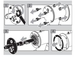
5 Place the burner insert in such a way that the insulators are protected against damage.
