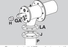
The nozzle set with NPT coupling is required for integrated ignition lances, see page 12 (Nozzle set).
