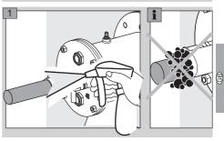
Avoid condensation due to the furnace atmosphere entering the burner housing. While the burner is switched off, at furnace temperatures above 500°C (932°F), it must be cooled with a low air volume - see page 9 (Cooling air).
