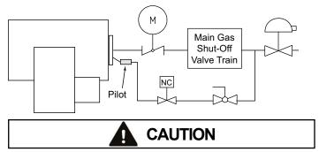
It is not possible to use a continuous or intermittent pilot. The pilot fuel flow should be interrupted after the trial ignition period has expired.
