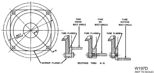
Figure 1. Three Typical Flange Mounting Arrangements
