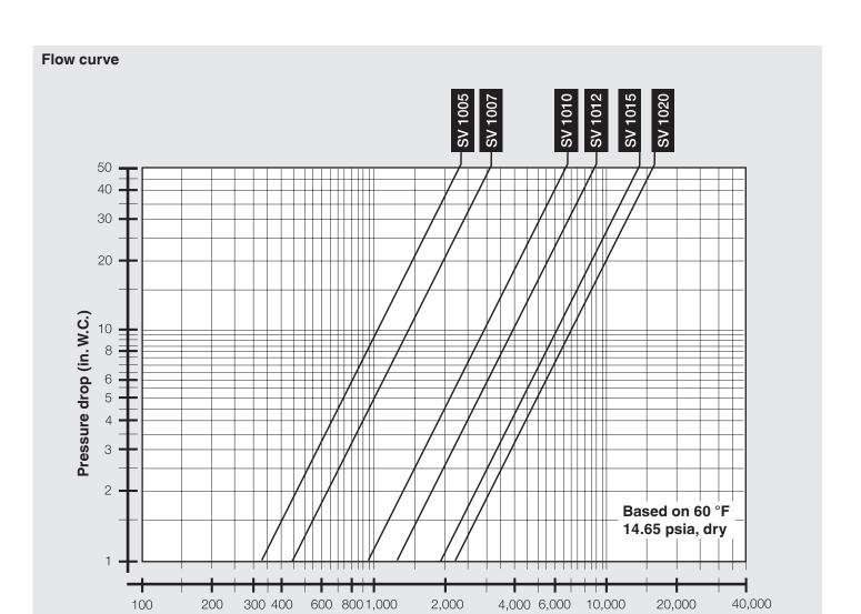
Flow (CFH) of natural gas; s.p. 0.65 at 60 °F
