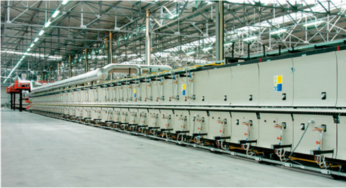
Ceramics industry: roller hearth kiln
