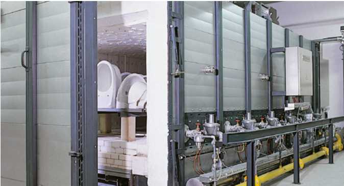
Ceramics industry: intermittent shuttle kiln
