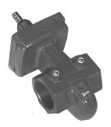
Normally-closed shut-off valves utilize power to open. Removal of electrical signal allows instantaneous release of the holding mechanism, allowing the powerful closing spring to close the valve in less than one second.
