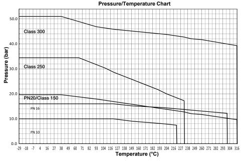
NOTE: Ratings are in accordance with ASME B16.4, ASME B16.5, EN 1092-1 or ISO 7005.
