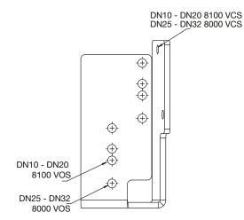
Figure 4: IP67 Switch Bracket
