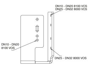
Figure 2: IP67 Switch Bracket
