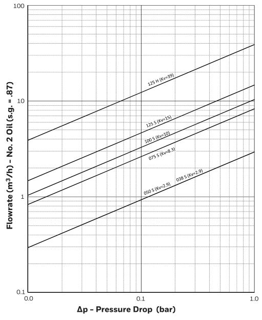
Maxon SSOV Liquid Flow Capacities
