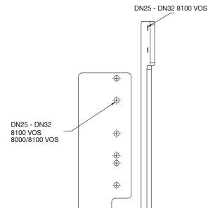
Figure 3: IP67 Switch Bracket
