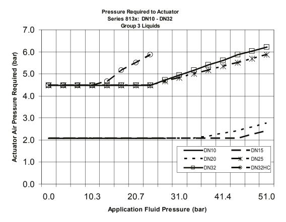
Group 3 fluids include: Liquid Ethanol, Liquid Methanol, No. 6 Fuel oil (heavy), Liquid Butane and Liquid Propane
