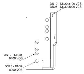
Figure 4: IP67 Switch Bracket
