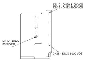
Figure 2: IP67 Switch Bracket
