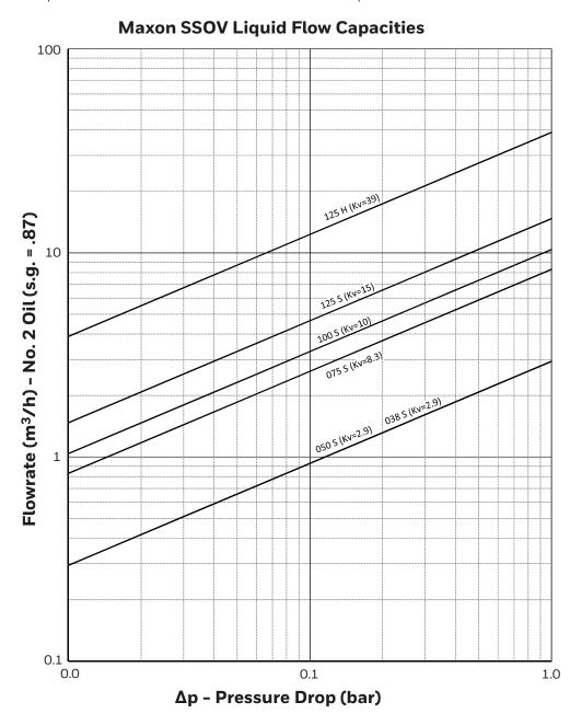
For preheated #5 or #6 oil, multiply the required flow rate in m<sup>3</sup>/h by the factor given in the table at right, then select a valve based upon that equivalent flow of #2 oil and the allowable drop.
