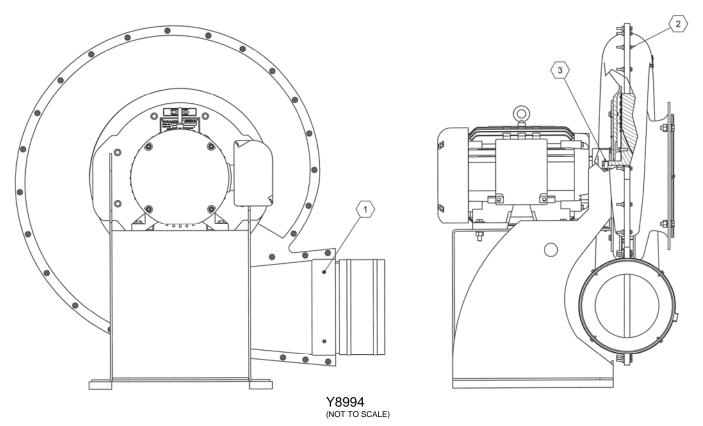
Figure 3. Typical Direct Drive Turbo Blower
