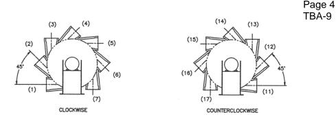
Figure 2. Standard Discharge Positions Viewed from Motor Drive End
