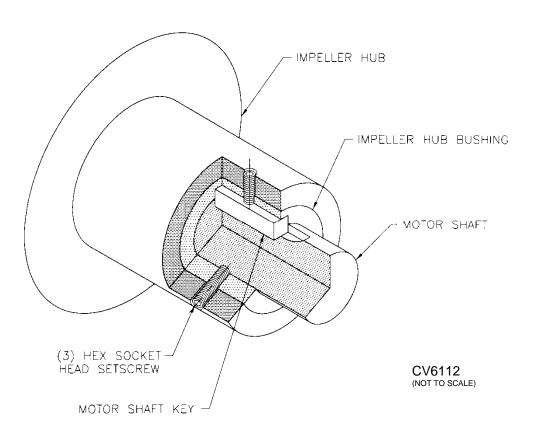
Figure 4. Blower Hub Locking Mechanism Cutaway
